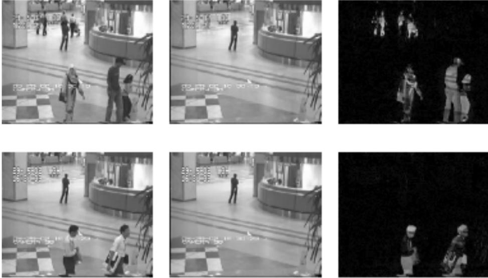
Figure 7: Surveillance video as low rank plus sparse matrices: Left = low rank (middle) + sparse (right). The background image leads to a rank-1 component and the occasional appearance of the customers contributes to the sparse component .
