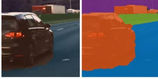
Figure 10: Autonomous driving. Clustering is used to help the system to identify and locate the vehicles and other objects on the road.
